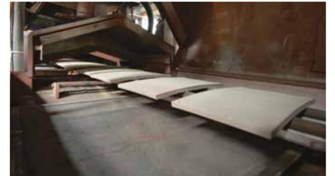
In addition to strict supply chain management, all unfired clay waste is introduced back into the production process which minimizes waste and maximizes the use of the raw material.
