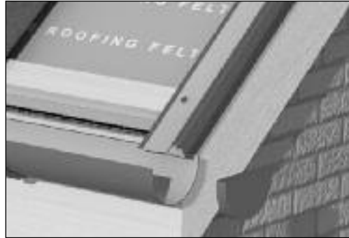
Fig. 1: Nail each length of trim to batten
